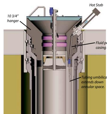
Cross-section of wellhead seal with mechanical mini-packer installed. A tubing umbilical in the space between the 16" and 10 3/4" casing terminates at the wellhead into a fluid manifold. The mechanism for hanging and sealing the 10 3/4" casing to the 16" casing with an internal tubing umbilical has been developed by IODP drilling engineers. A Hot Stab is shown connected to the fluid manifold.
