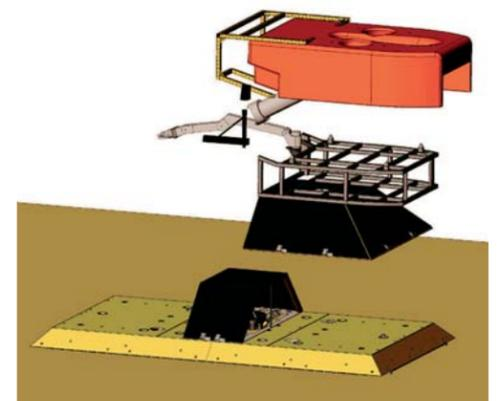
A mockup illustrates the use of the Recovery Stab and an ROV to lift a science module off the wellhead template. A small hydraulic winch installed in the ROV's toolsled is used to secure the science module against the underside of the toolsled. This Recovery Stab was originally designed for the MARS (Monterey Accelerated Research System) submarine cable installed in Monterey Bay in 2007.
