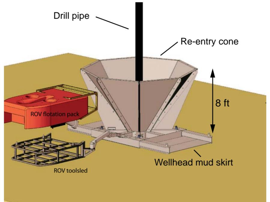
This schematic diagram shows the existing re-entry cone wellhead design used by the ODP and IODP. A full-scale mockup of MBARI's ROV Ventana is shown without its mid-section to reveal more of the wellhead. This re-entry cone is not ROV friendly or trawl-resistant. The mudskirt supports standard IODP casing hanger assemblies (3 or 4 Drill Quip casing hangers).
