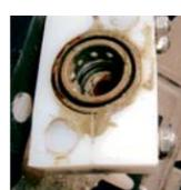
Test shows effects of 4 month exposure of an off-the-shelf quick connector to seawater. Non-corrosive materials are required for a 10-year useful life.
